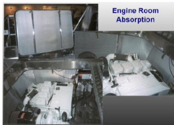
Figure 2 Use of MM in engine room for absorption in marine applications
